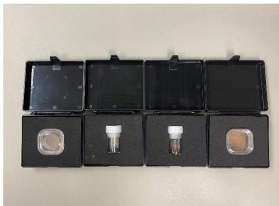
Image 4 and 5: HKU Department of Earth Sciences is currently home to these lunar samples, which were collected by China's Chang'e-5 lunar probe in 2020 and weigh a total of 822.6 milligrams.
